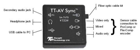
Connect the sensor to the PC using a USB cable. This powers the sensor and carries sound signals from the PC
