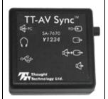
The TT AV-Sync sensor is a highly accurate time-synchronizing device for making measurements of audio and video events produced by a PC. The TT-AV Sync is used in evoked and slow cortical potential protocols, and reaction time testing to provide measurements with millisecond accuracy.
