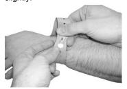
Connect cables as shown. Cables can also be connected to the electrodes before placing the straps.
