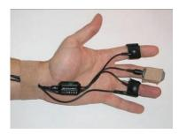
Also note that, in this image, a blood volume pulse (BVP) sensor is connected to the middle finger, although BVP is not included in the Reaction Time suite.
