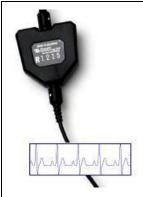
The EKG sensor is a pre-amplified electrocardiograph sensor, for directly measuring heart electrical activity. It connects via extender cables for a single channel hook up.
